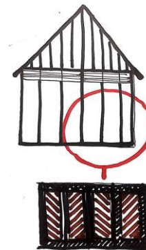
Figure 2.1(d): sketch of the half timber infilled with herringbone brickwork and stucco
